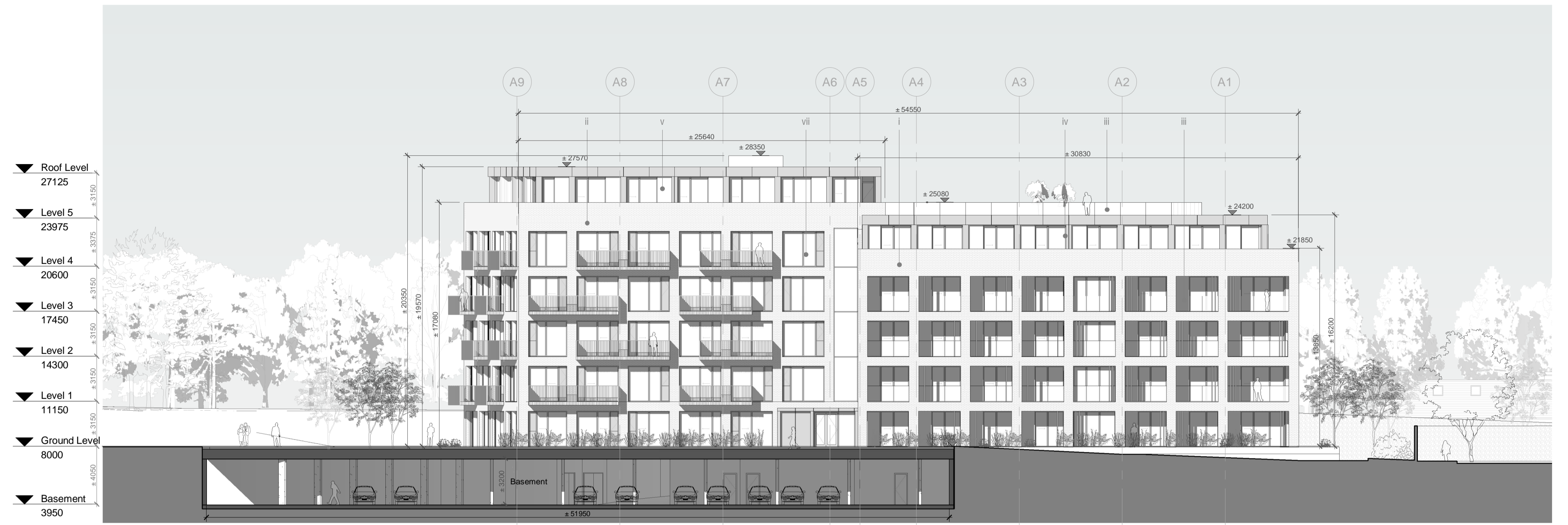
2 Building A - East Elevation scale 1 : 200
